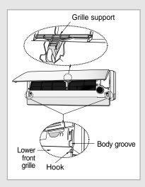
For the best use of your air conditioner, you must clean it every two weeks regularly to remove the dust that accumulates on the air filter.
